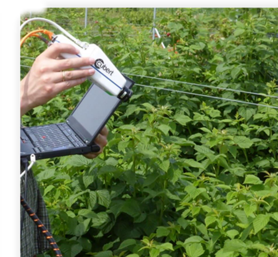
Image acquisition with Cubert Cam
