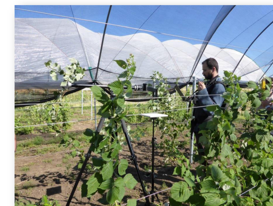
White reference measurement under black cover material
