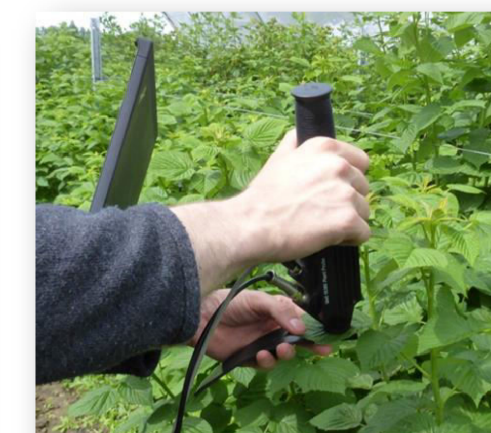
Spectral sampling with Contact Probe
