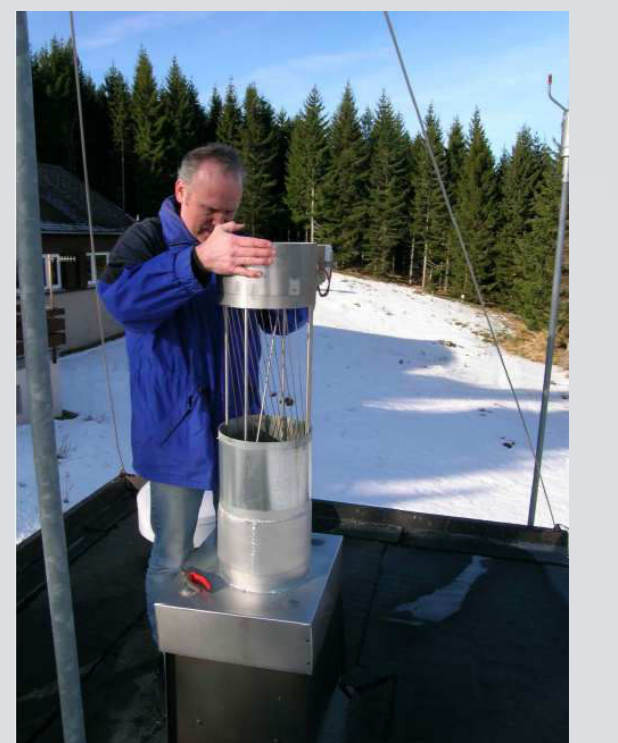
Insertion of inlet tube heating DEP33 (RASA)
