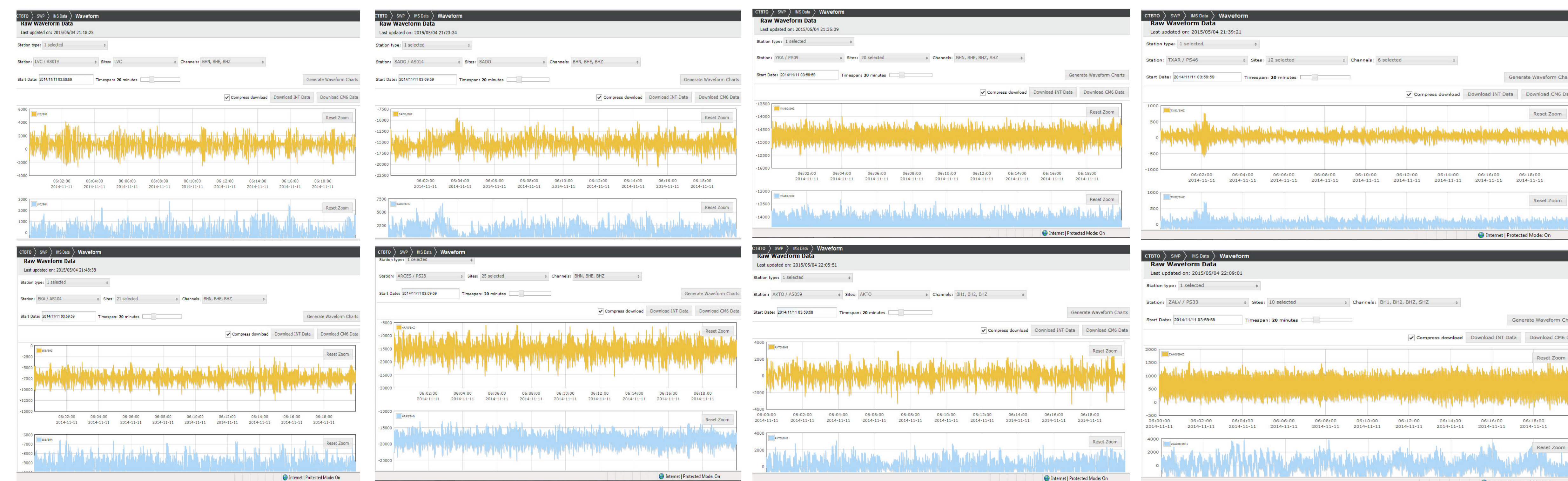
Figure 2 below shows screenshots of IMS waveform data from different seismic stations as requested by CTBT Support on the 13/11/2014 6:54 PM. The waveform data shows a systematic two hours time shift.
