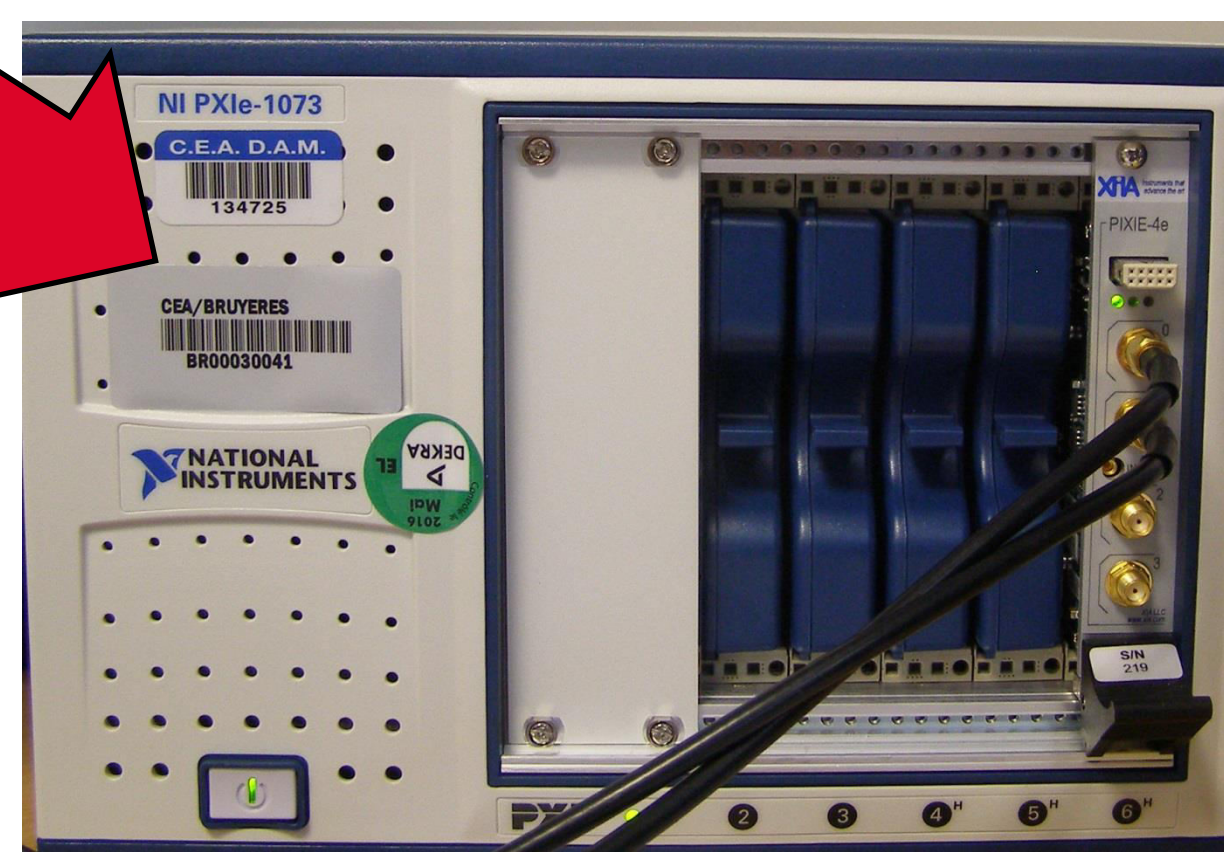
Analogue electronics used to record HPGe energy in anticoincidence with a cosmic veto
