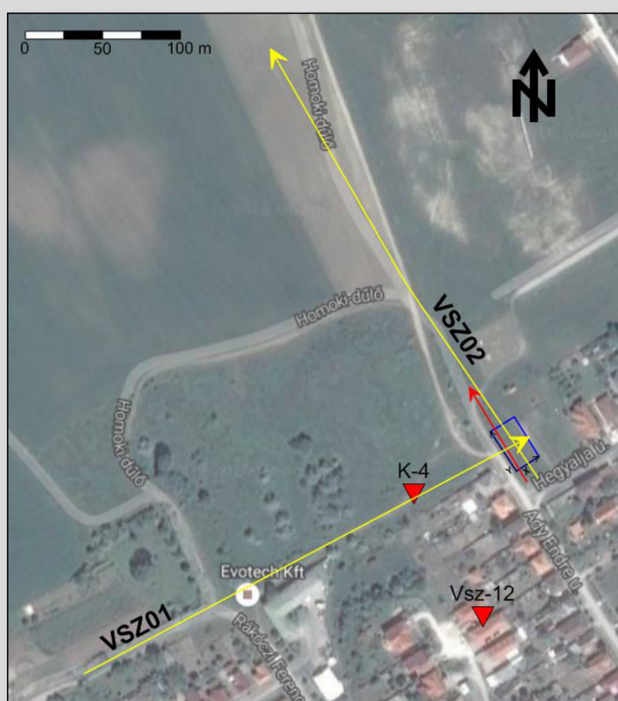
Fig. 2. Location of the geophysical surveys: 2D geoelectric lines (yellow), S-wave seismic line (red) and 3D geoelectric layout (blue). Red triangles are borehole locations
