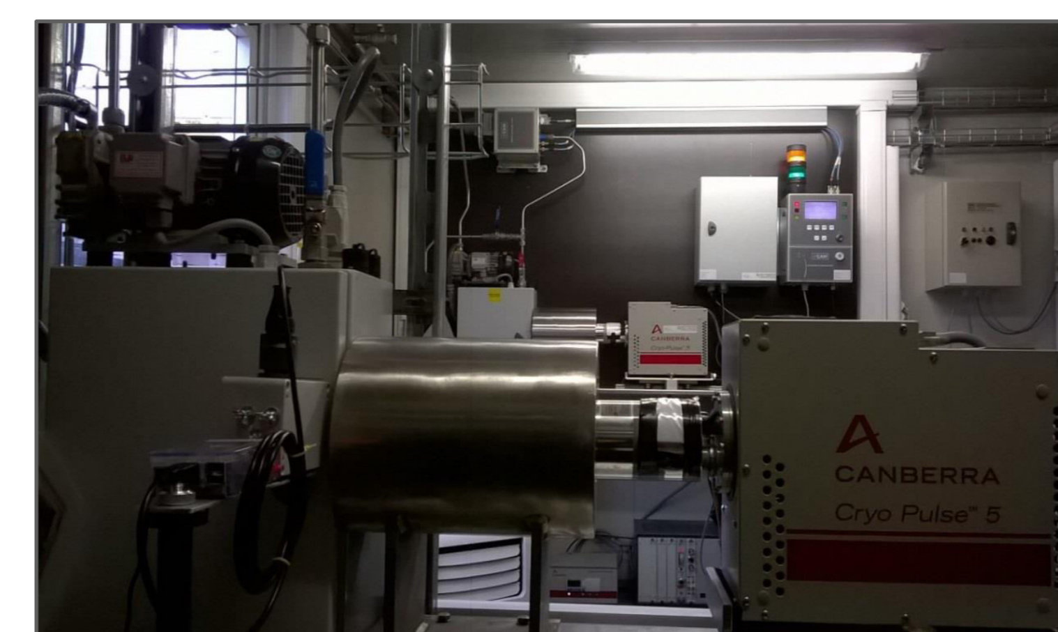
Fig. 3 – The two monitoring systems running in parallel: the main system using charcoal in the background, the secondary system using silver zeolites in the foreground.
