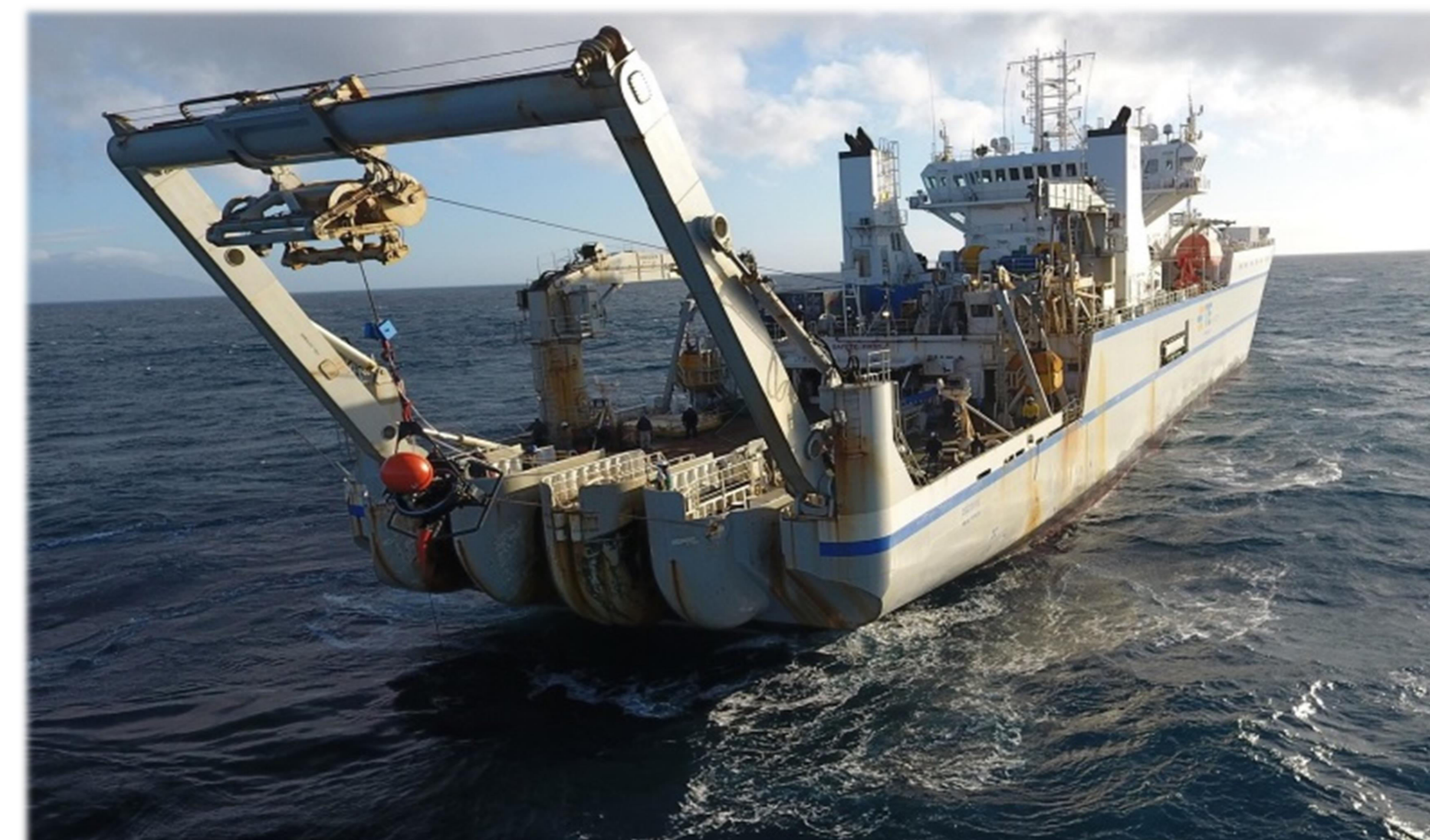
Figure 4. The overboarding of the last node/hydrophone of the North HA04 triplet from the cable ship C/S Decisive on the evening of the 29th December 2016, photographed from a drone.
