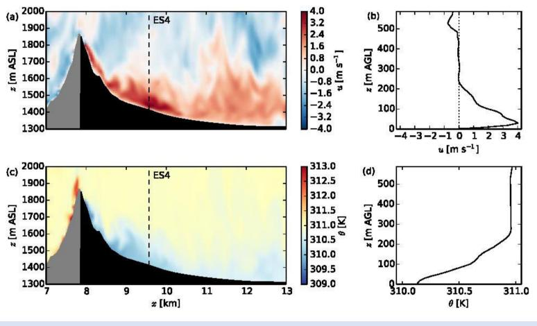
In a cross section through the green dots, which represent measurement towers from the MATERHORN field experiment, the characteristic jet structure of the downslope flow can be seen.
