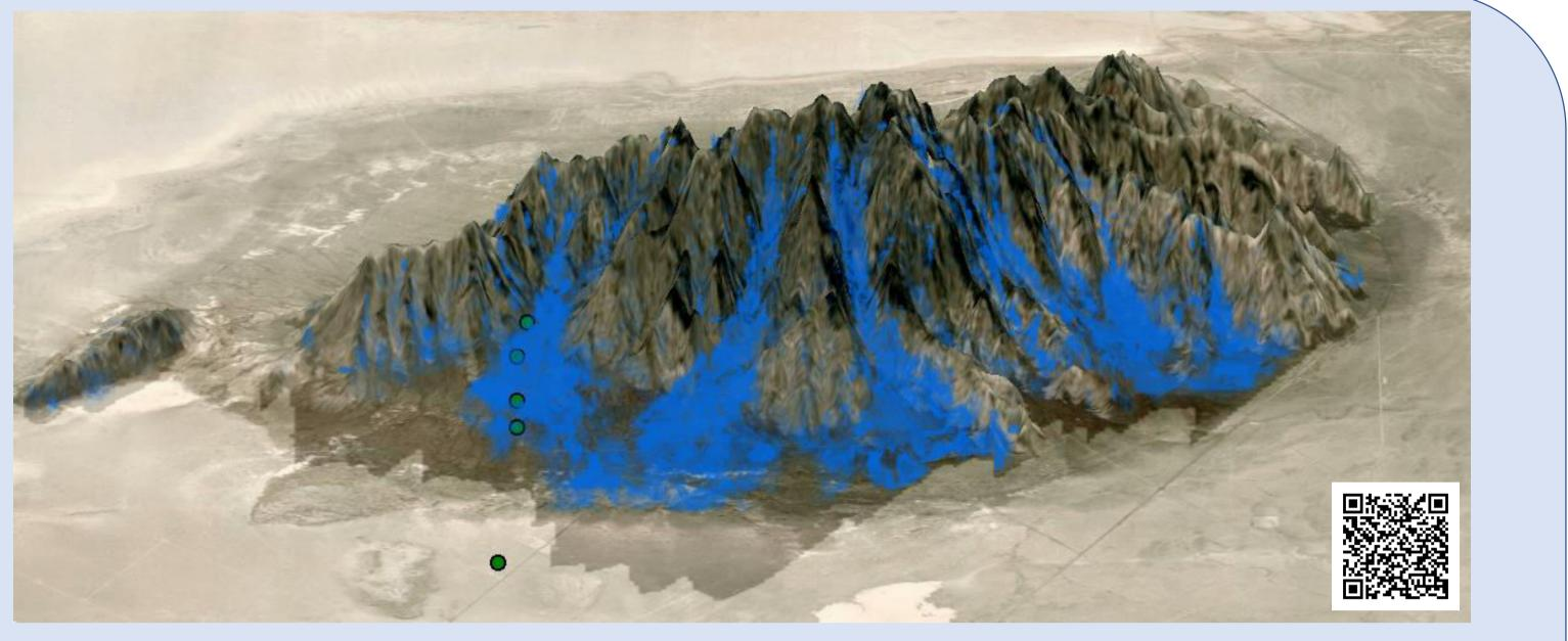
The image above shows isosurfaces of downslope velocity from the model at 18:55 MST. Darker blue surfaces represent faster flow. The terrain is shown by a real satellite image from Google Static Maps API. Topographic shading is shown as well. Follow the QR code to a watch an animation of the modeled downslope flow as it develops.
