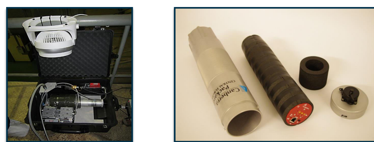
Fig. 2 – Experimental setup as initially installed at BATEK and exploded view of the detector, housing, thermal insulation and OSPREY.
