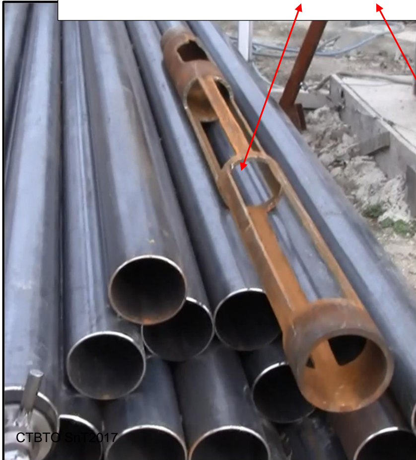
Slotted dilatometer installation casing
