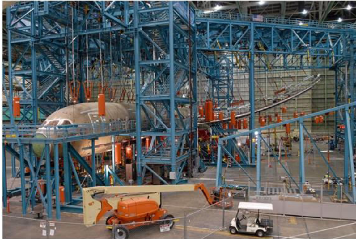
Boeing 787 Full Scale Structural Test Specimen
