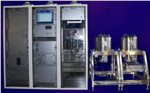
The SAUNA xenon monitoring system uses adsorbent separation along with beta-gamma detection
