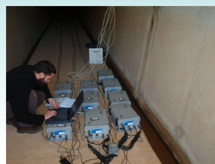
CGS short-period stations operation test in KEDDARA dam; on the left, Kinemetrics K2 digitizers, on the right, Lennartz LE-3DLitt sensors (50 cm apart from each other).
