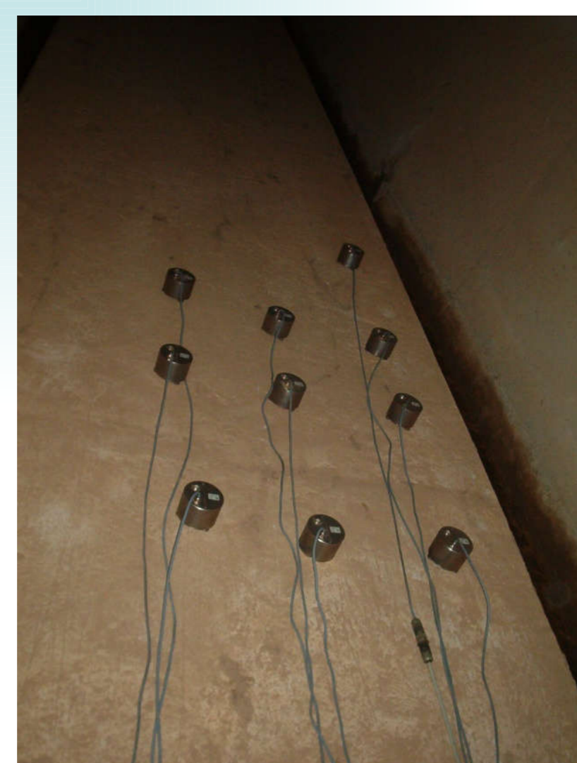
CGS short-period stations operation test in KEDDARA dam; on the left, Kinemetrics K2 digitizers, on the right, Lennartz LE-3DLitt sensors (50 cm apart from each other).
