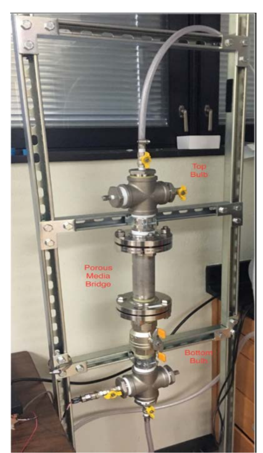
2-bulb gas column located at UT Austin
