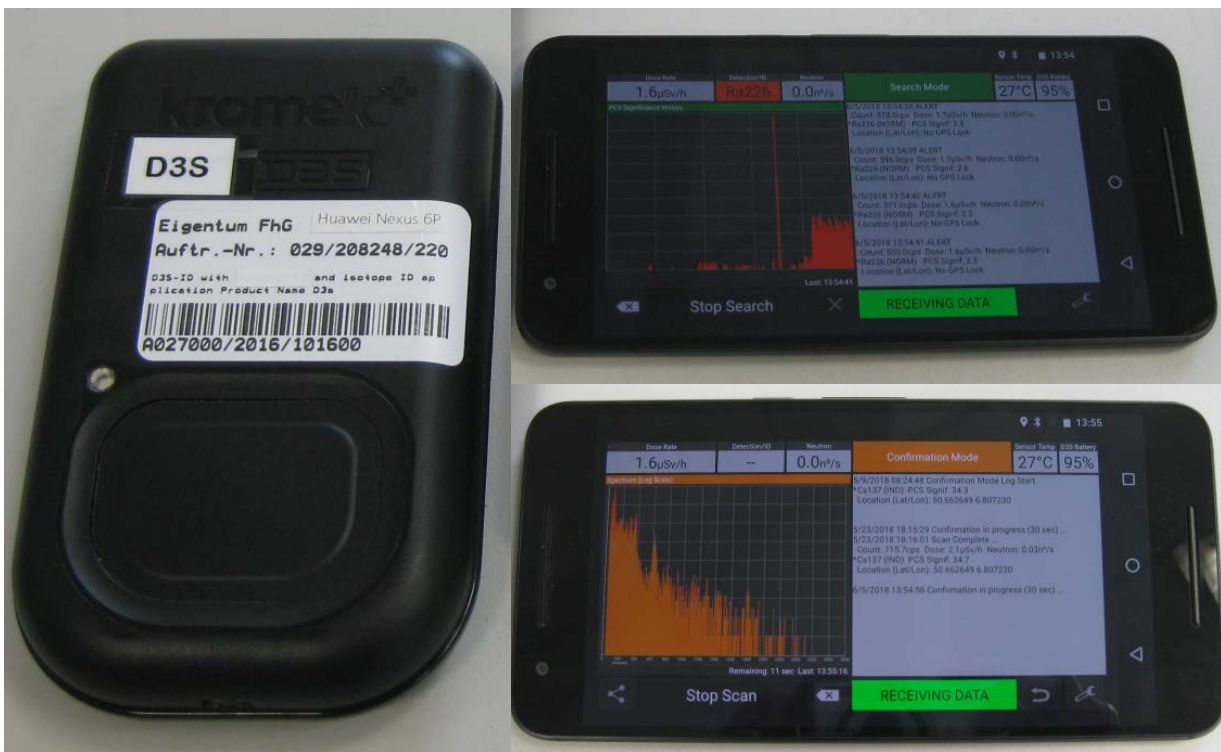
Fig.3: D3S Pictures of the D3S detector (left) and the display device in both modes.
