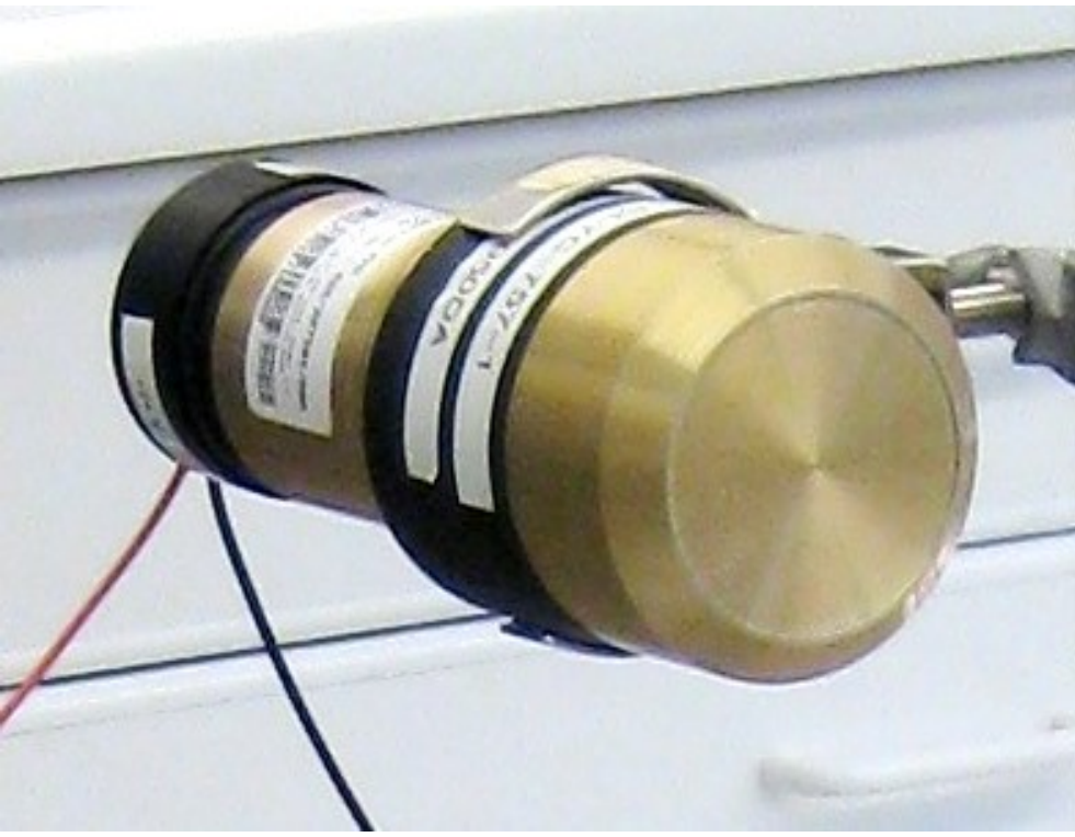
Fig.5: CLYC Picture of the CLYC detector with base.
