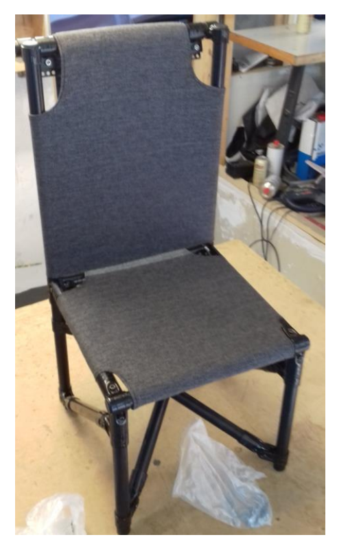
A four point harness was developed and fitted to each chair. It was considered important to demonstrate to trainees the reduced movement possible when such a harness is used as opposed to a conventional lap belt.
