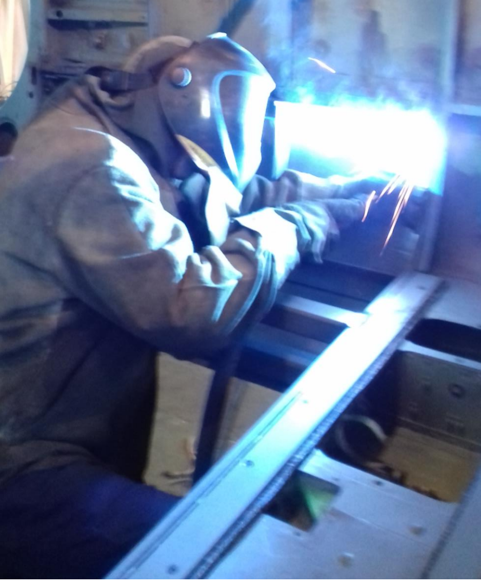
In contrast a normal airframe, structural components in the simulator could be welded in place. Once complete, a false floor could be added (right).
