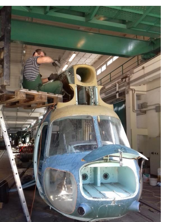
On delivery, the airframe was stripped of any unnecessary components such as the platform in the central portion of the cabin. Essentially the airframe was reduced to its skeleton to enable the customisation for OSI requirements.
