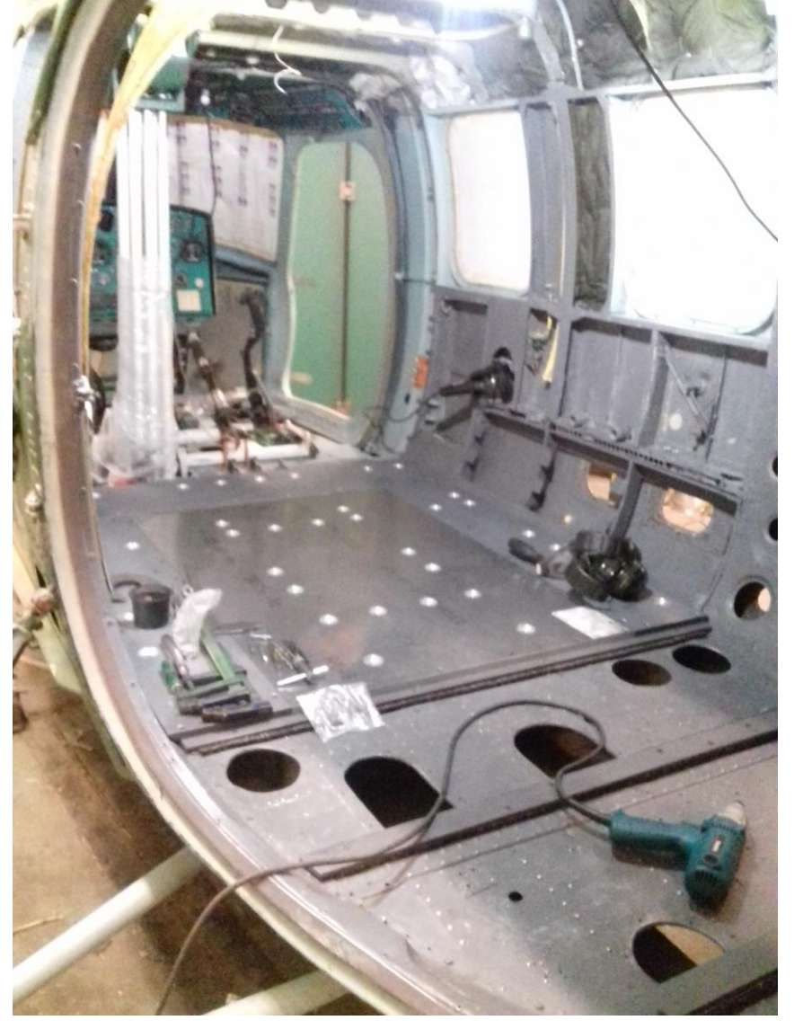
In contrast a normal airframe, structural components in the simulator could be welded in place. Once complete, a false floor could be added (right).
