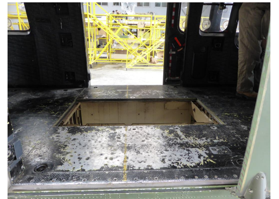
On delivery, the airframe was stripped of any unnecessary components such as the platform in the central portion of the cabin. Essentially the airframe was reduced to its skeleton to enable the customisation for OSI requirements.
