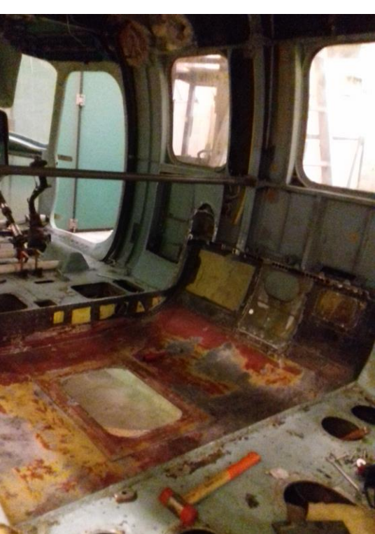
On delivery, the airframe was stripped of any unnecessary components such as the platform in the central portion of the cabin. Essentially the airframe was reduced to its skeleton to enable the customisation for OSI requirements.
