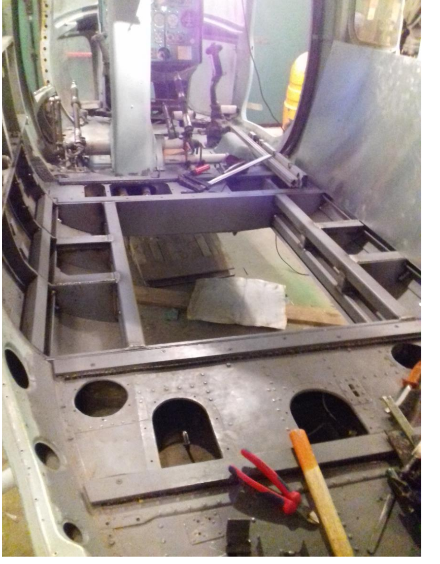
In contrast a normal airframe, structural components in the simulator could be welded in place. Once complete, a false floor could be added (right).
