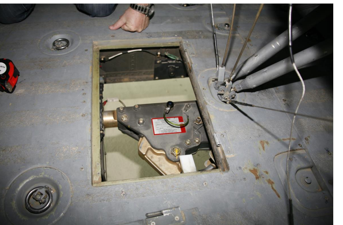
The Sikorsky UH-60 Black Hawk also has an internal hatch but considerably smaller than the AS232
