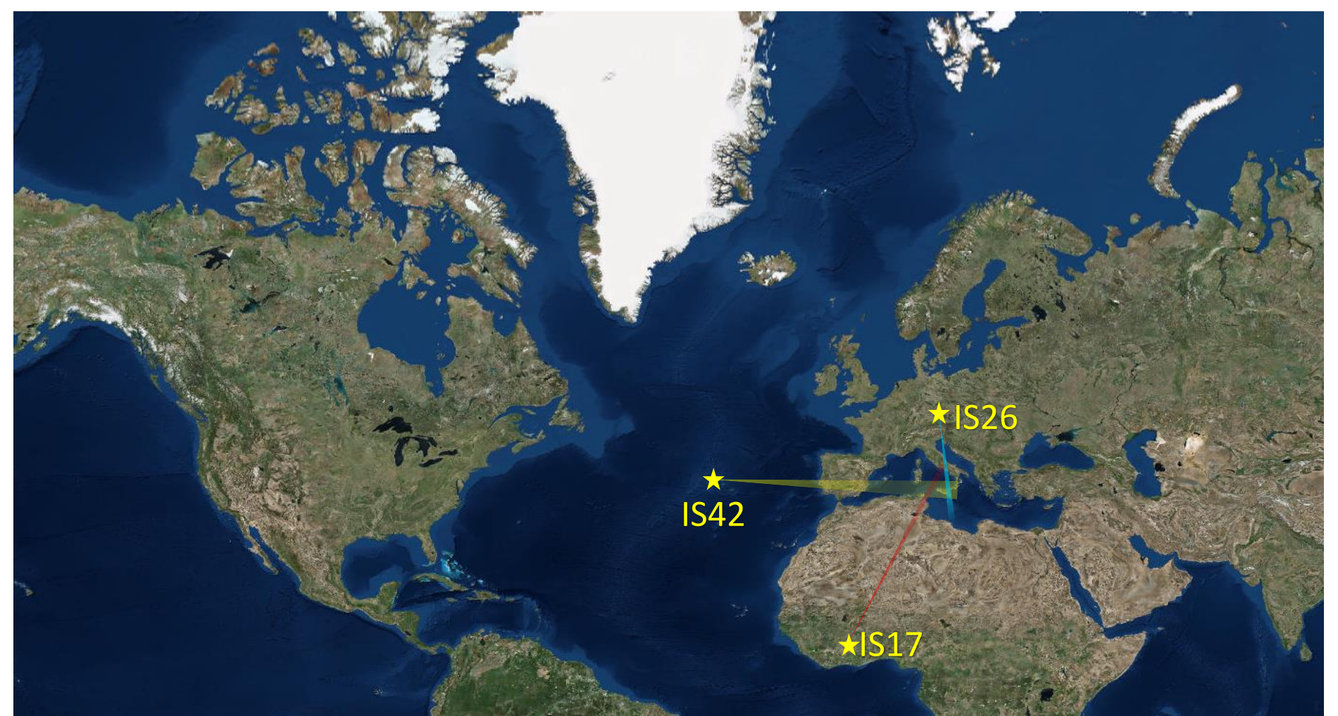
Figure 4 - Illustration of the mean back-azimuths range for all the events recorded in each station.
