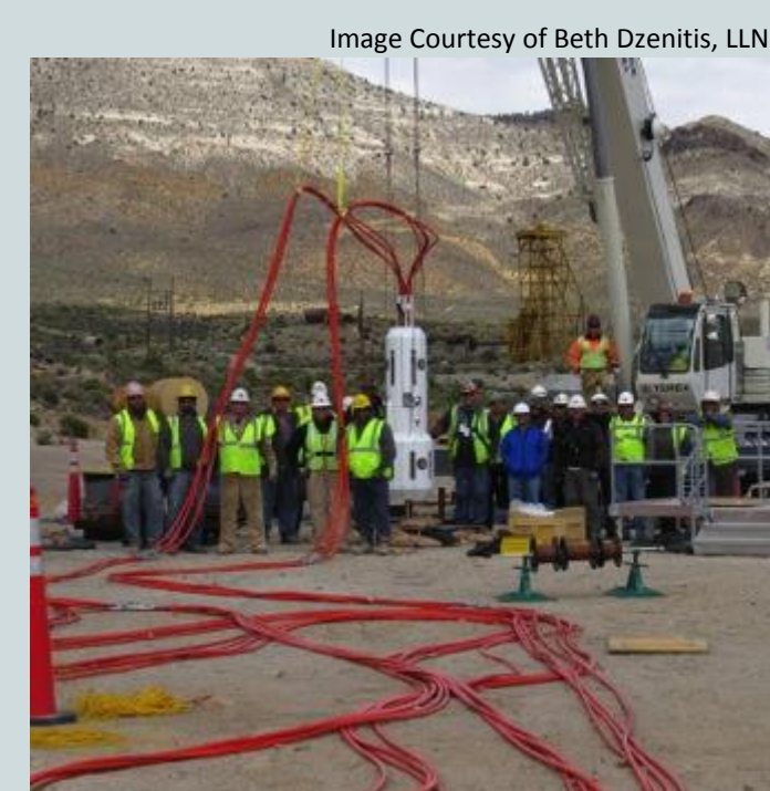
Emplacing a SPE chemical explosion canister (0.2 tons)
