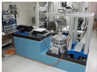
CEA infrasound sensors calibration with the new laser pistonphone
