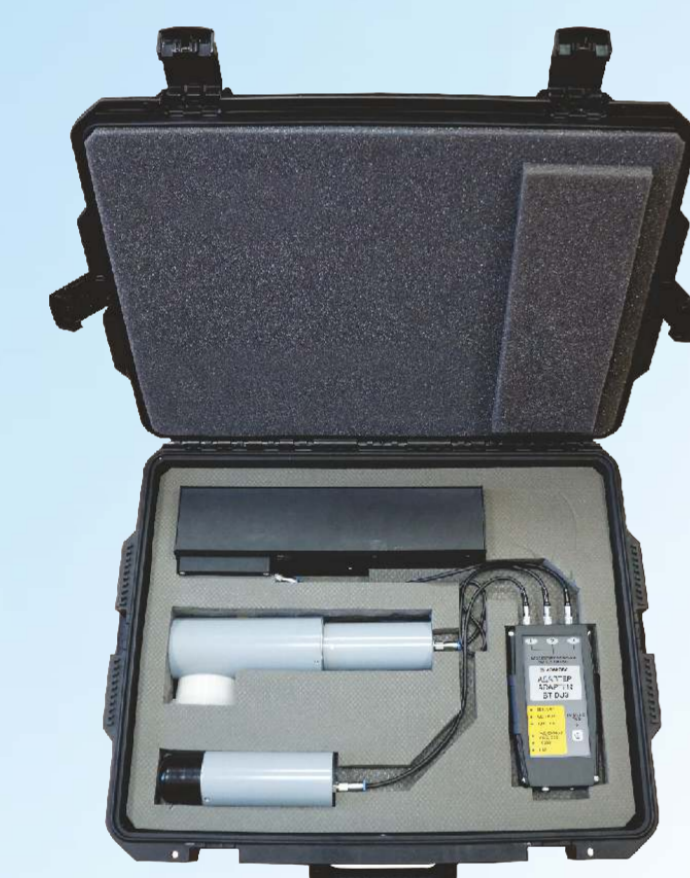
Gamma radiation and neutron radiation monitor: BDKG-11M (1 unit), BDKG-04 (1 unit), BDKN-05 (1 unit)
