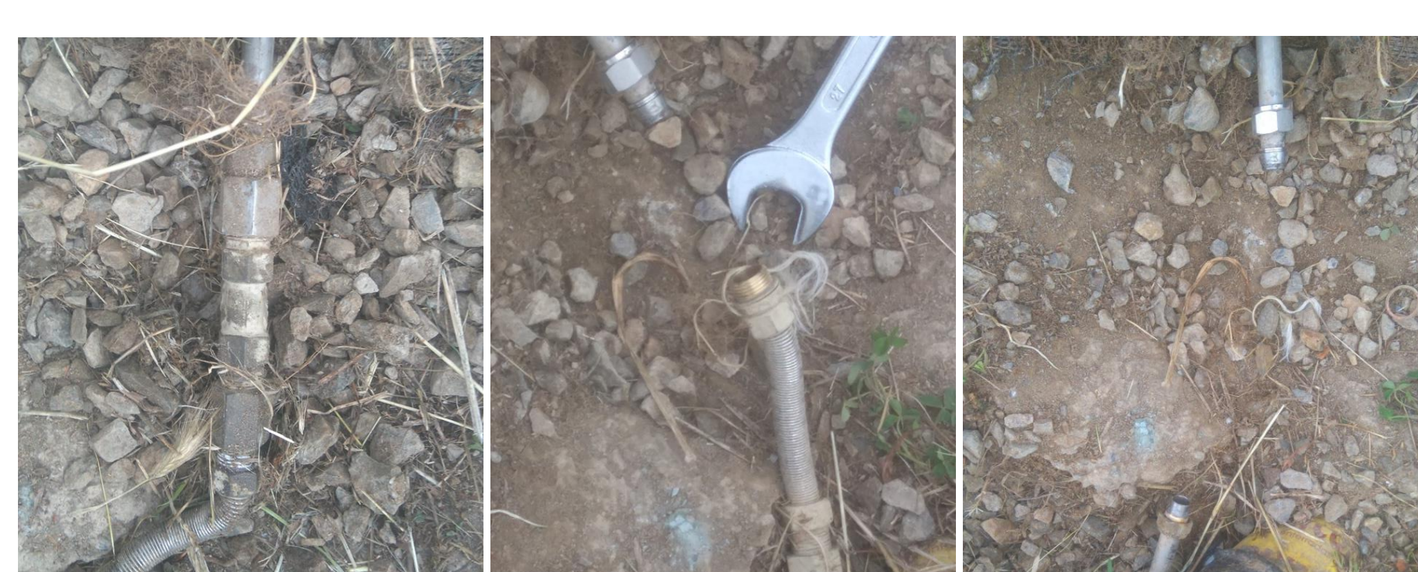
Flexible pipe and resonance suppressor of main line connected to micro barometer dry.
