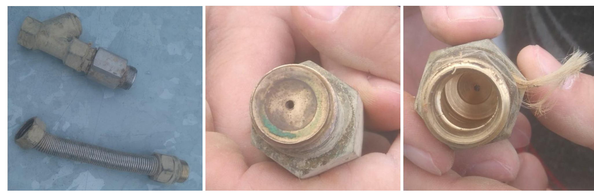
Flexible pipe and resonance suppressor of main line connected to micro barometer dry.
