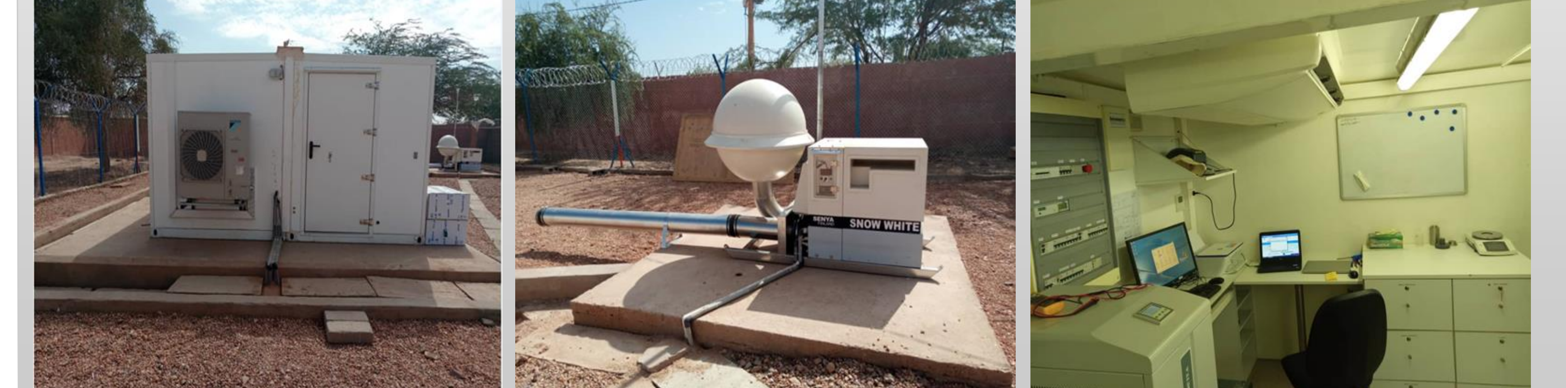
Local of the station NR48 Station RN48 air sampler system inside the station RN48
