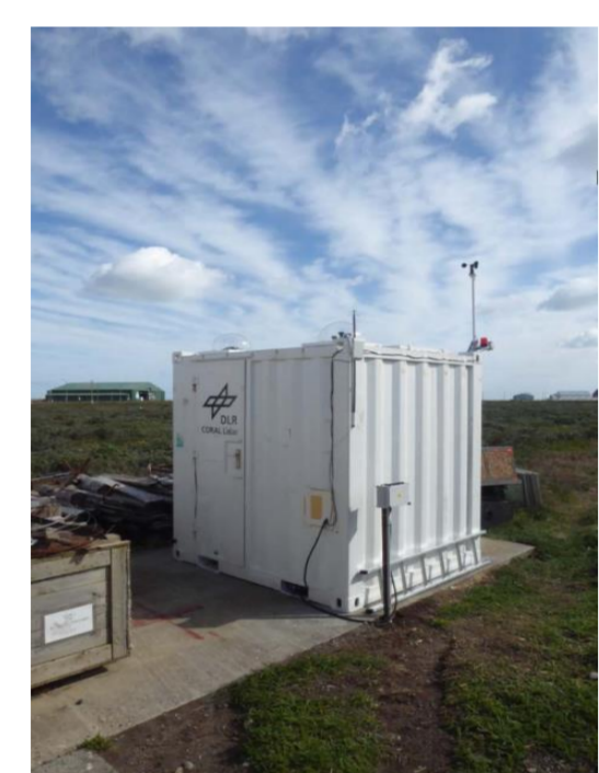
Fig. 1: The CORAL lidar collects backscattered laser light (532 nm, 14 W power, 100 Hz repetition rate) by a 70 cm telescope in three height-cascaded channels. It is integrated into an 8-foot container at EARG station in Rio Grande and operates autonomously using local weather data and forecasts.
