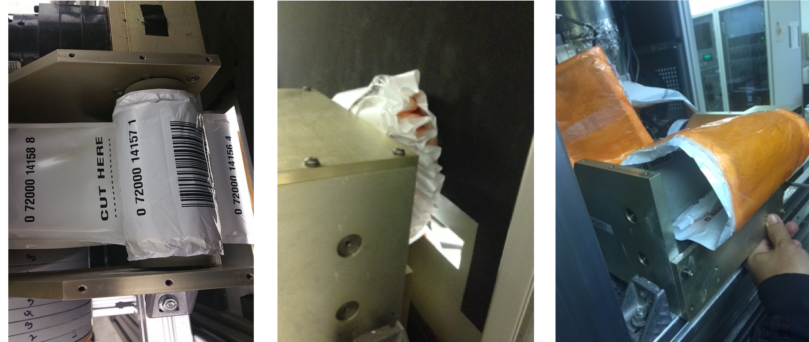
RASA Filter Jams – Wrapped around Rollers, Stuck inside Panels, and System Disassembly for Recovery
