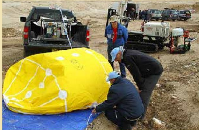
Soil-gas sampling for noble gas detection.
