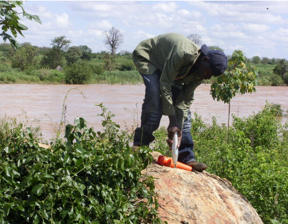
T2.2-O1: A rapid and non-destructive method for determining in-situ UCS of rocks during OSIs
