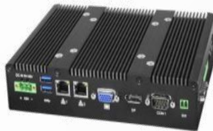
Industrial PC -40°C to 70°C, Intel CPU, Win10
