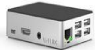
Raspberry Pi 3 B+ ARM, Linux
